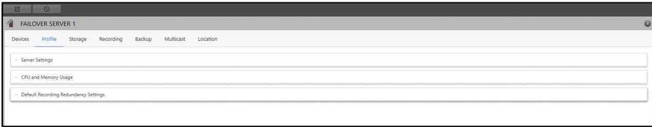
The Profile tab contains three collapsible panels — Server Settings, CPU and Memory Storage and Default Recording Redundancy Settings.
