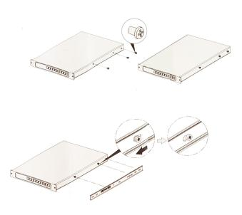
Fasten it with the P-head to make sure it is well locked and the inner rail does not loosen from the system.
