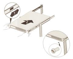
• You can use Round Hole pins or Square hole pins. Align the holes of the system with those of the rack and insert the screws. Tighten them to fix the system in place.
