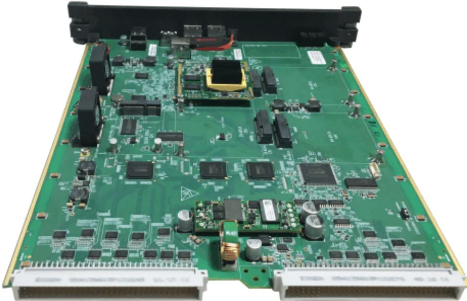
You may install the second NX DBM VOCODER64 Module by locating the **VOIP #2** label on the CPU board and follow the same steps as above. Similarly, install the other modules if required.
