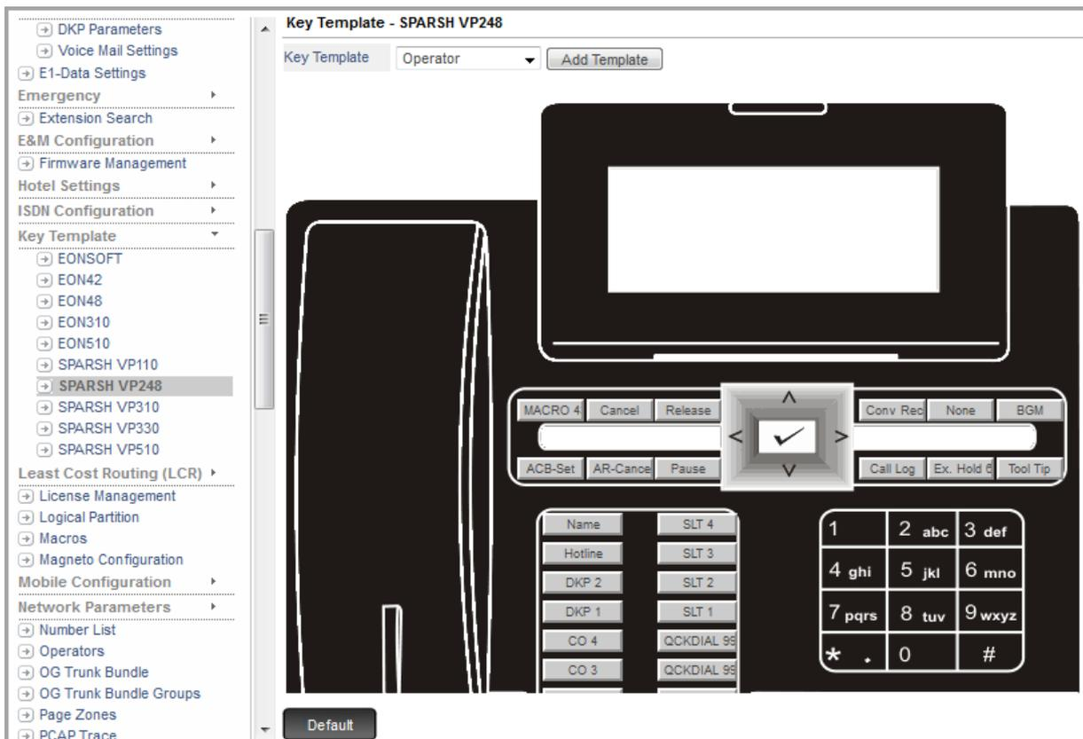
For example, to customize the key template the keys that need to be reassigned features are as follows:
