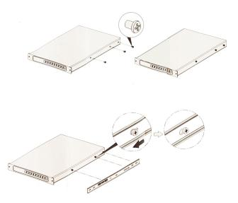
• Fasten it with the P-head to make sure it is well locked and the inner rail does not loosen from the system.
