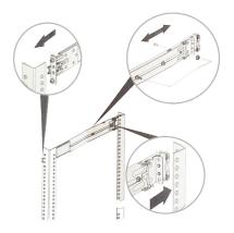
• Make sure the bearing retailer in locked forward. Horizontally install the system half way into the slide rail.
