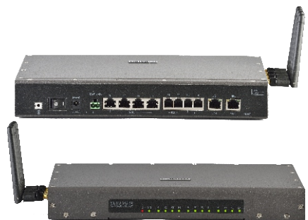
SETU VGRX Radio-over-IP Gateway with Integrated GSM/CDMA Connectivity
