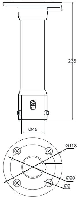
Fig.3.2.2 Picture of dimensions of ceiling installation arm
