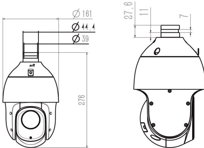
Fig.3.3.3 V3 HD infrared network high speed dome camera dimensions specification
