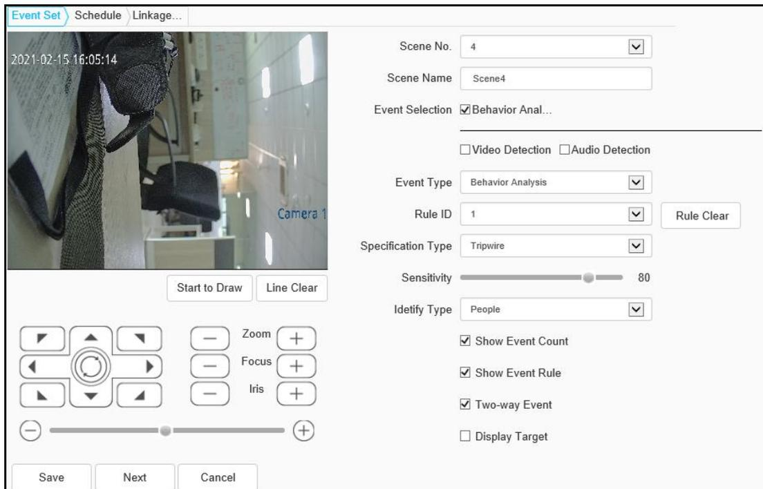
Fig.5.12.1.2 tripwire setting interface
