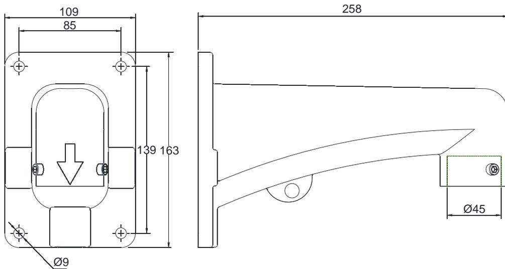
Fig.3.2.1 picture of dimensions of wall-mounted installation arm
