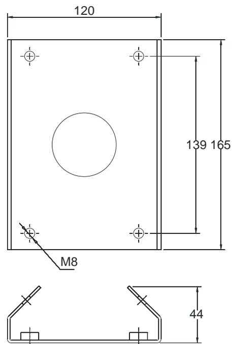
Fig.3.2.4 Picture of dimensions of column-like installation arm
