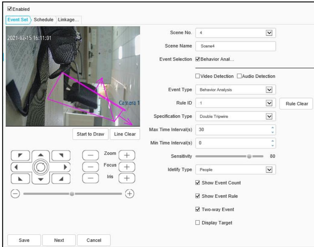
Fig.5.12.1.3 double tripwire setting interface
