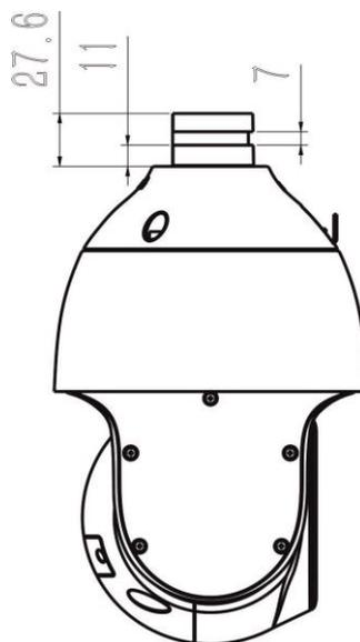
Fig.3.3.4 Picture of dome camera and interface dimensions
