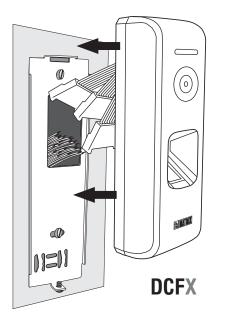
2. Align COSEC PATH on mounting plate and slide it downwards as shown below.
