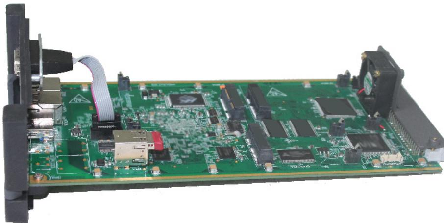
This card hosts Communication Manager, Feature Server, VoIP Server, VMS Server and other important servers and modules which controls all other slave cards (SLT, DKP, CO+SLT, DKP+SLT, E&M, BRI, T1E1, E1FO, GSM/CDMA etc.). All the configuration and programming information is stored on this card.
