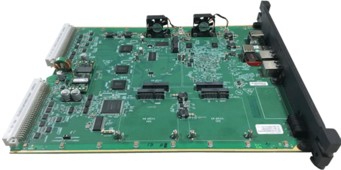
This card hosts Communication Manager, Feature Server, VoIP Server, VMS Server and other important servers and modules which controls all other slave cards (SLT, DKP, CO+SLT, DKP+SLT, E&M, BRI, T1E1, E1FO, GSM etc.). All the configuration and programming information is stored on this card.
